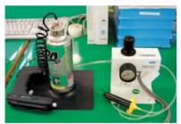
Replacing the Use of the Old Spray-can Propellant (left) by the Use of Air (right)
